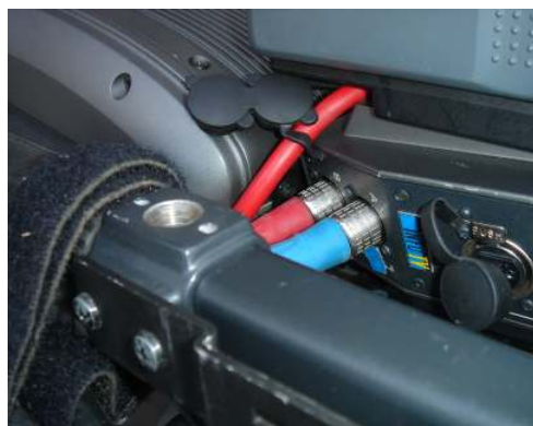
The handle in L hinders the connection Dual Link
