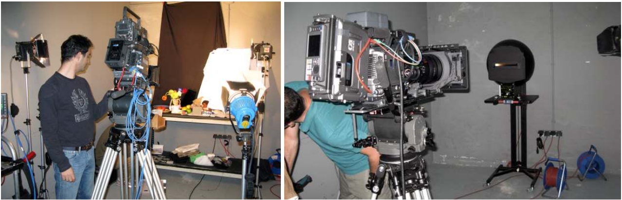
Images of the test room at Info Tv during a still life shot where we can see the different configurations of the camera. Also shooting the Stouffer Transmission Step Wedge mounted on a light sphere. In the picture, Ramiro Sabell, First Assistant Camera.
