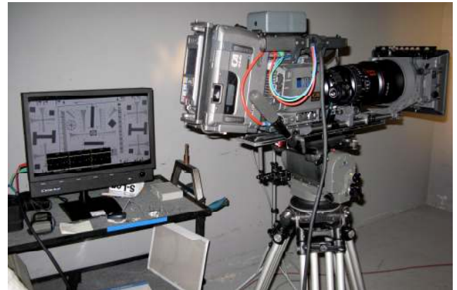
Evaluation of ISO chart in test room of INFOTV.
