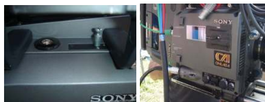
Pivot to mark the focal plane and gadget on the camera for holding the decameter.
